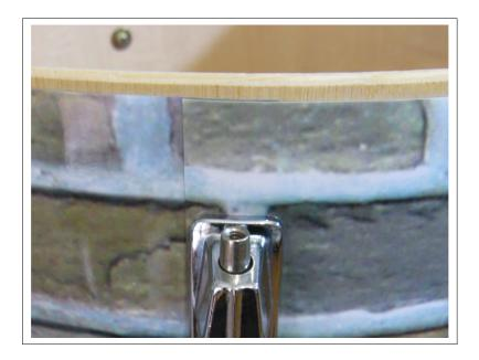
The wrap is placed around the shell, securing its edges with the spring clamps. An effective method to make it adhere properly to the shell is to slide multiple times with the fingers along the entire circumference, repositioning the clamps each time, until a snug fit is achieved. If the shell is already drilled, you need to make sure that the overlap corresponds to the lug holes.
