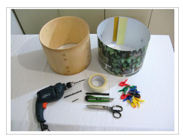
DrumStroke's trimmed wraps are usually supplied with two strips of double-sided adhesive tape applied on the back (unless the customer requires a different installation method). The strip marked with number 1 will be attached directly on the shell; the strip marked with number 2 is of a high strength type and will be attached partially on the shell and partially on one edge of the wrap, creating an overlap.
