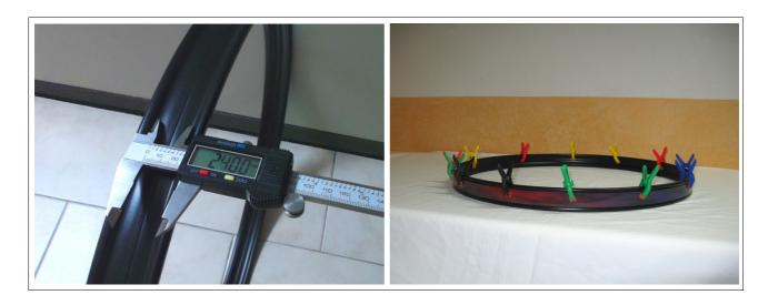
The wrap is placed around the hoop, securing it with plenty of clamps.
