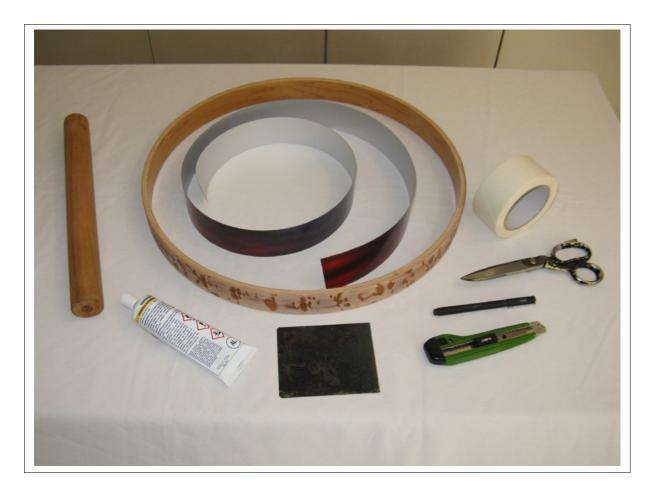
The external surface of the hoop must be cleansed of all residues of previous paint or glue jobs that could chip off. In the example of our photos we used a hoop whose original wrap was removed with indelicate methods, leaving dents in the surface, and then painted. We sanded the paint, obtaining a regular enough surface, though without completely eliminating the dents.
