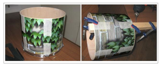
If, instead, the shell is already drilled, the existing holes will act as a guide. With a sharp nail or screw you pierce the wrap, from the inside to the outside, keeping the shell on a relatively soft surface like old newspapers or corrugated cardboard. It might be helpful to tap lightly with a hammer. Using these small holes as a guide, the actual holes are made with the drill.
